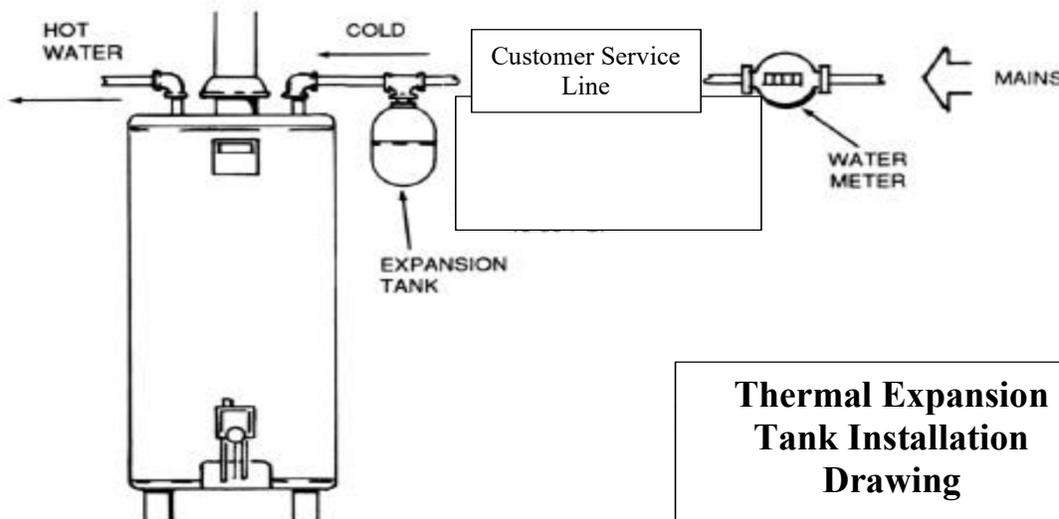
**Thermal Expansion Tank Installation Drawing**
